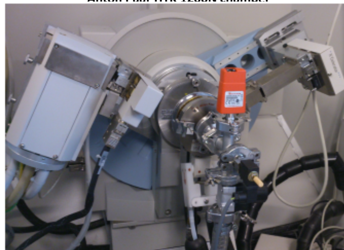
Sample in the low temperature Anton Paar TTK 450 chamber
